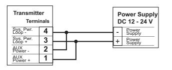
Connection to a PLC/Recorder, separate supply
